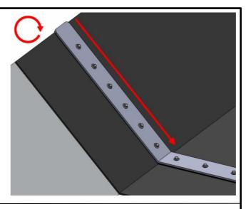
**Perform a final check** of the tension in each fixing. Make any adjustments you deem appropriate.
