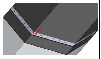
Fix the Strip to the base of the gutter, working inwards from either side towards the centre.
