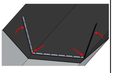
Chose a side and **press the upstand** down **onto the gutter's side**.
