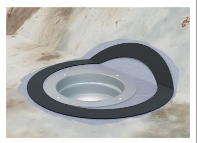
Install the Plygene Liner over the outlet.
