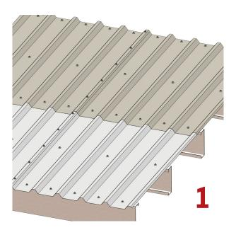
Ensure the roof/area/fixings to be treated are clean and free from debris and dirt. (Removal may be carried out using a pressure washer fitted with a rotating spinning head capable of delivering a minimum of 3000 psi.)
