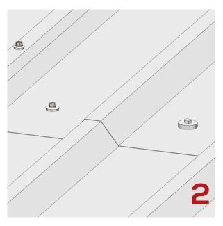
Ensure all fixing caps have been removed and rust suitably prepared.
