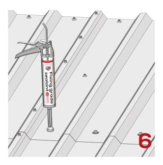
Place nozzle over the fixing, ensuring it is flat and level. Squeeze the trigger ensuring that required amount of sealant dispenses to encapsulate the fixing.
