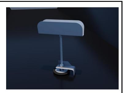
Working about the centre, turn the Cutting Tool Anti-Clockwise (Blunt Edge Leading) to score a circle into the liner.
